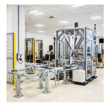
Delta robots are used for applications where fast operations are required. Developed in cooperation with industrial partners, this five-axis Delta robot in Testbed enables synchronization of its movements with the movement of the pallets on the conveyor. Researchers designed and finetuned a kinematic and dynamic model to compare the behaviour of a real robot with the expected ones and to identify differences through machine learning algorithms.
