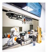
In addition to the two collaborative robots, the Robobar in Testbed for Industry 4.0 also uses the functions of other devices, including a liquor conveyor, fruit feeders, an ice feeder and more. It's all connected via a common industrial communication platform.
